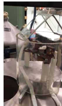
After plating was complete, the plates had a cloudy look. The material needed to be crystallized in order to readily pass light through them. The plates were removed and taped together with Kapton® high-temp tape, making sure to have the scintillation chemicals in between them and a gap between the half-plates that is large enough to allow a fiber in between.
