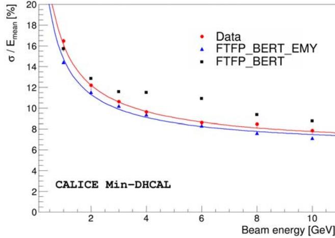
**Figure 3.** Energy resolution versus positron beam energy for data (red) and simulation based on FTFP (black) and FTFP\_BERT\_EMY (blue). The experimental points were corrected for the known momentum spread of the beam. The error bars of the data include both statistical and systematic uncertainties. The error bars of the simulation indicate the statistical uncertainty only. The curves are the results of fits to the quadratic sum of a constant and stochastic term.
