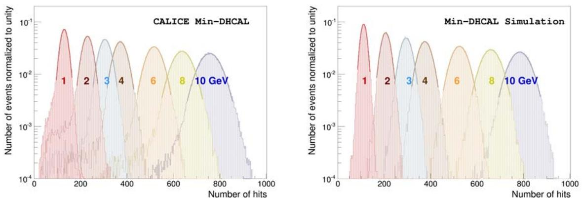
**Figure 1.** Distribution of the number of hits for all selected positron events for data (left) and simulation based on the FTFP\_BERT\_EMY physics list (right). The distributions are plotted separately for each beam momentum setting (1, 2, 3, 4, 6, 8, 10 GeV/c) and are each normalized to unity. The distributions are fit with a Gaussian function in the range of  $\pm 2$  standard deviations. The results of the fits are shown as solid lines.
