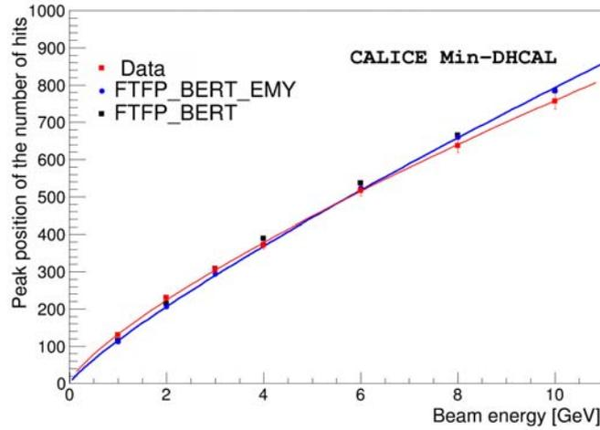
**Figure 2.** Peak position of the number of hits versus positron beam energy for both data (red) and simulation based on FTFP\_BERT (black) and FTFP\_BERT\_EMY (blue). The experimental data points and the simulation based on FTFP\_BERT\_EMY have been fitted to a power law shown as solid lines. The error bars of the data include both the statistical and systematic (dominant) errors. The statistical error bars of the simulation are smaller than the marker size.
