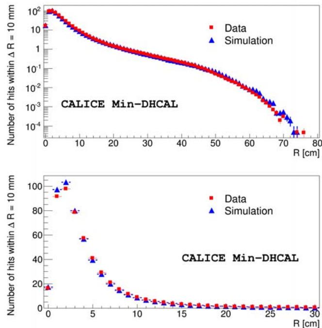
**Figure 4.** Distribution of the radial distance of hits from the shower axis for 6 GeV positrons. The upper (lower) plot uses a logarithm (linear) y-scale. The areas of both plots are normalized to one event. The error bars include the statistical and systematic uncertainties for the data and statistical uncertainties only for the simulation.
