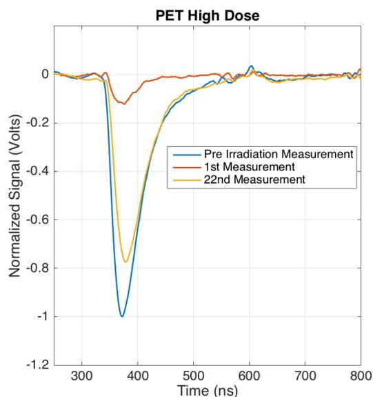
**Figure 2.** Average waveforms of the pre irradiation measurement, the 1st measurement immediately after irradiation, and the 22nd measurement after irradiation, taken over 40 days of the PET 14 Mrad dosed sample.
