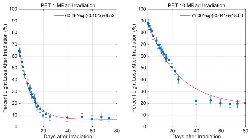
**Figure 4.** PET Results, 21 measurements over 40 days.
