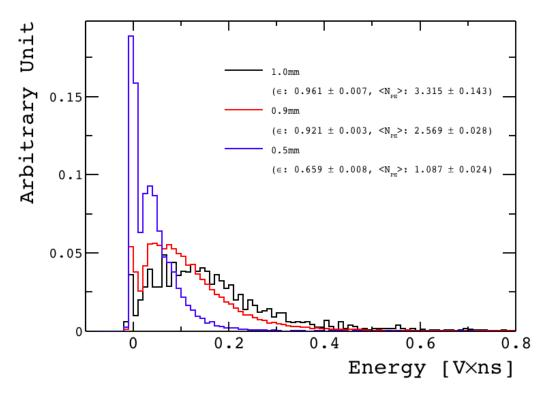
**Figure 5**. Comparison between the light output of liquid scintillator tiles readout with plastic WLS fibers with different thickness. The light output, proportional to the energy released by a particle traversing the scintillator volume, is measured in units of photodetector pulse area. The three distributions are normalized to have the same area of 1.
