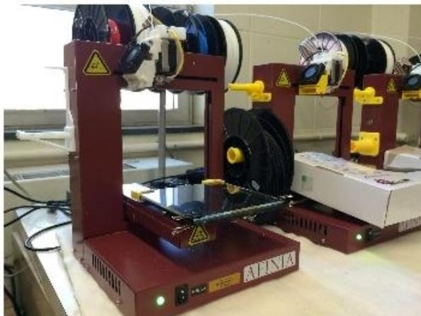
**Figure 1.1** Afinia H480 3D Printer displays the Afinia logo along with a status light to indicate power and operation, and an initialization button to ready the machine to print. In the rear of the machine shown in *Figure 1.3*, a 19V power supply input and
