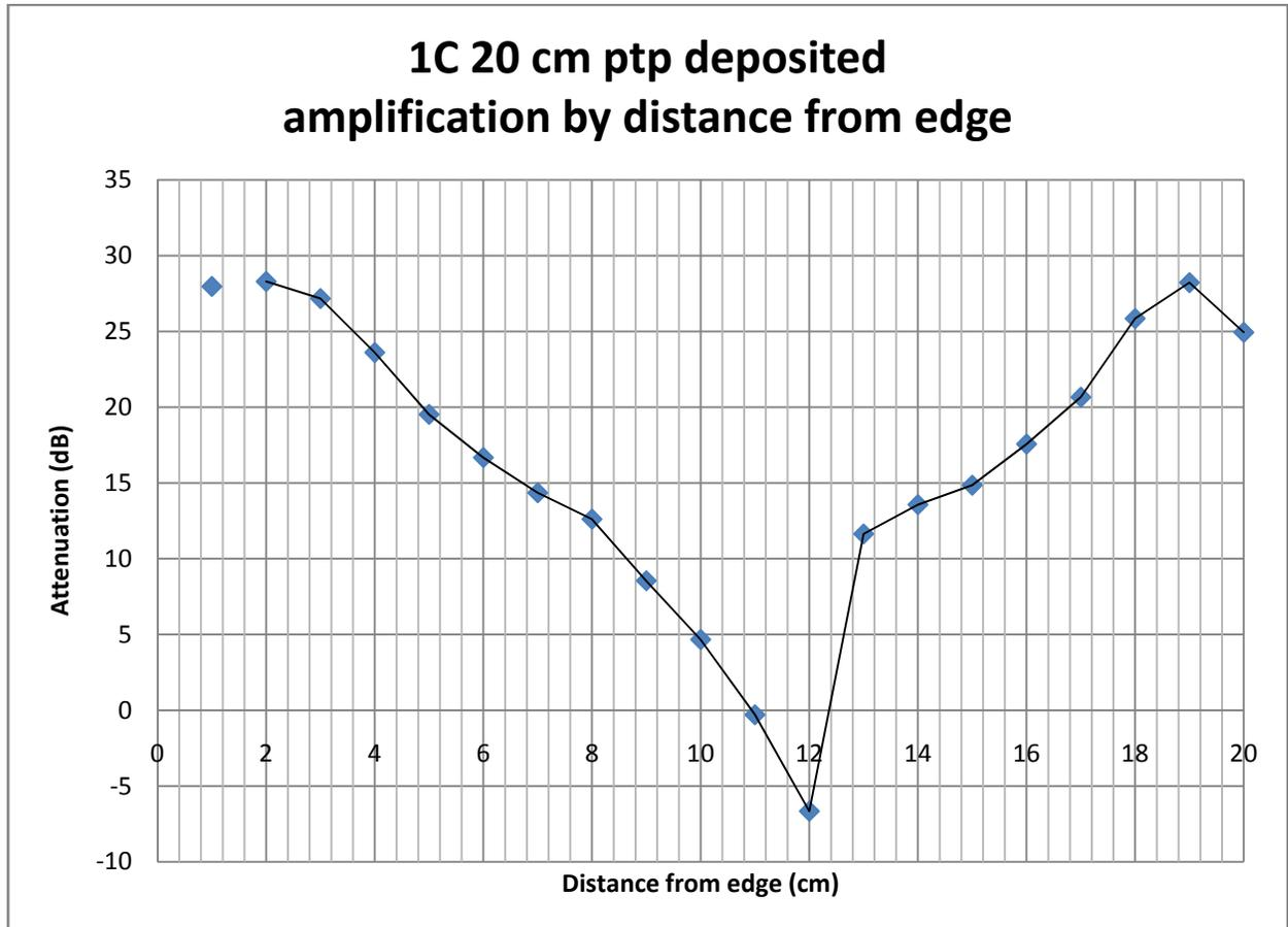
This is the graph of amplification in dB vs. distance from edge for the 20 cm treated area. It seems the symmetry of our fiber setup is a bit off but the graph appears to show that there is considerable fall off from about 3 to 4 cm widths. Perhaps this is our maximum fiber width that gives the best active area to fiber loss.
