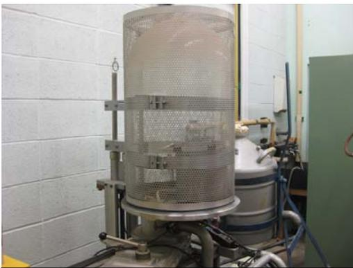
PTP deposition in the vacuum chamber
