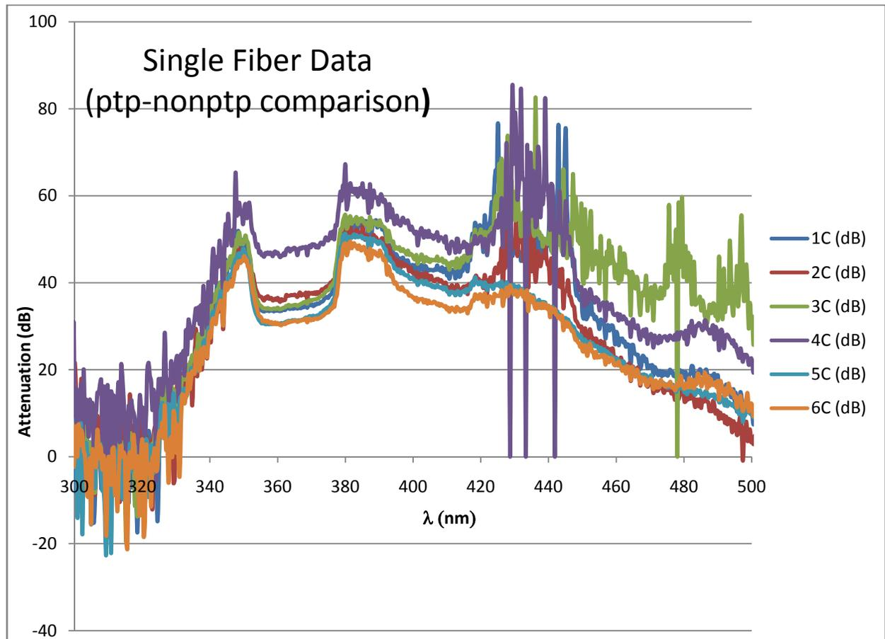
This graph indicates the margin of noise to be approximately  $\pm 20$  dB. As one can see, configurations 3C and 4C seem to have the best amplification of light from their baselines, particularly in the 400 to 500 nm range. 5C and 6C seem to have less than the 20 cm configuration.
