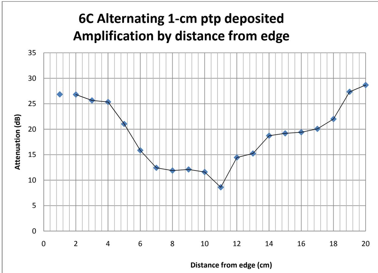
This graph shows the distribution of attenuation over the distance edge-to-edge for the 1 cm-staggered treatment. It appears to have higher signal than the bare 20 cm width but still suffers from loss in the center but to a lesser degree.
