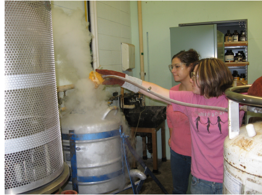
Teacher Moira Truesdell (left) and Brittany add liquid nitrogen to the diffusion pump trap.
