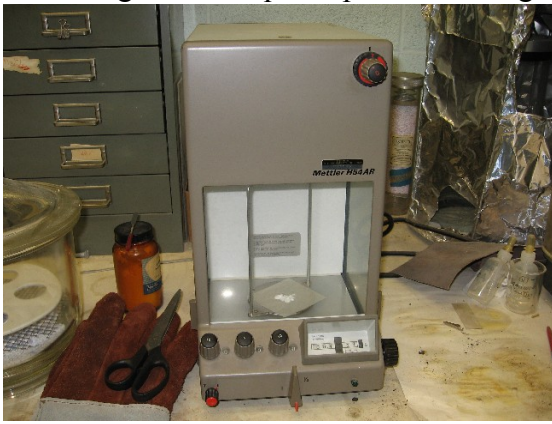
Analytical Balance used for PTP measurement
