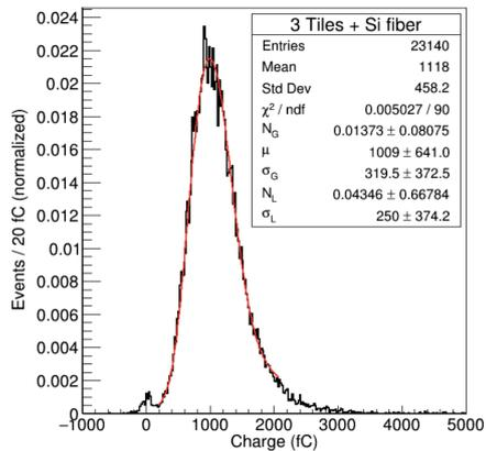
**Figure 7.** The charge distribution and the fit to Gaussian + Landau for the response of the 3 tiles + fiber assembly to 150 GeV muons.
