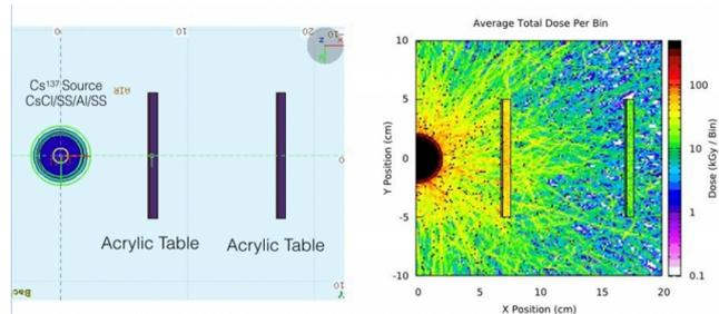
**Figure 2.** The displays from the Fluka simulation of the radioactive source and the sample holders.
