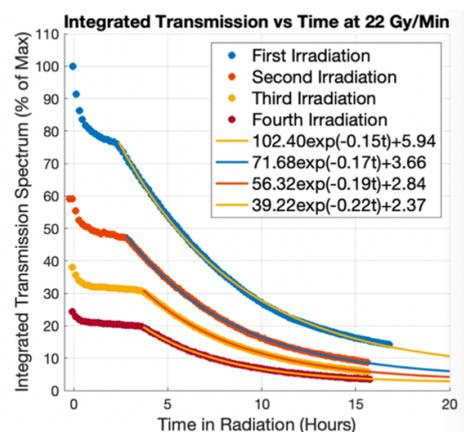
Fig. 5. The integrated transmission vs. time for the four consecutive irradiation campaigns for the blue fiber.
