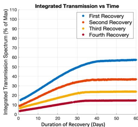
Fig. 7. The transmission spectra integrals as a function of duration of recovery for the blue fiber.
