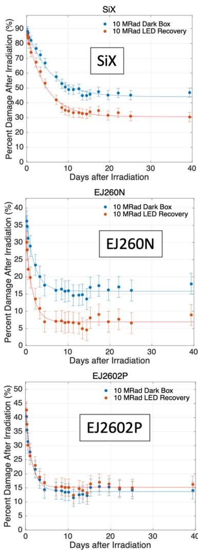
Fig. 3. Percent damage after irradiation for Scintillator-X (top), EJ-260 (middle) and EJ-260P (bottom) for 40 days following irradiation.
