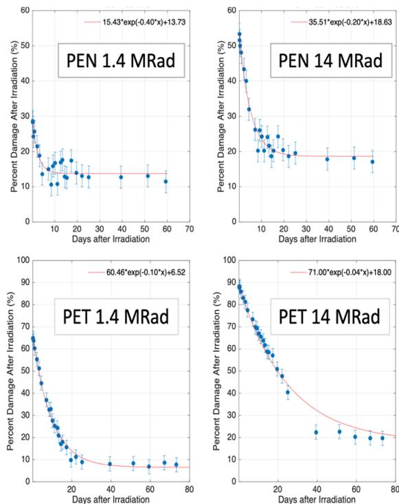
Fig. 2. Percent damage after irradiation for PEN (top) and PET (bottom) samples that were irradiated to 1.4 MRad (left) and 14 MRad (right) for a duration of approximately two months.
