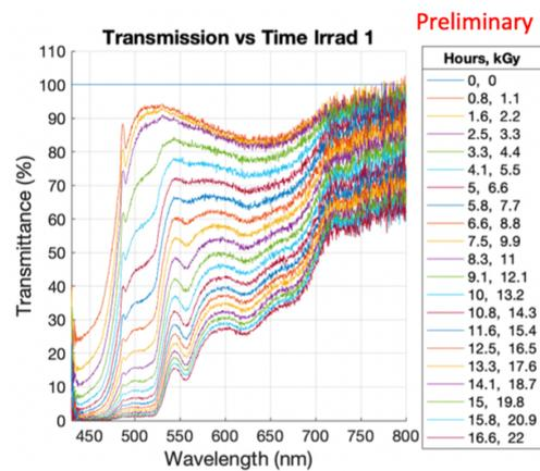
Fig. 4. The transmission spectra of the blue fiber as a function of irradiation duration.
