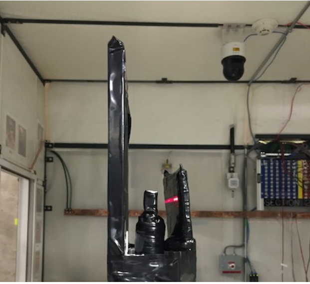
Fig. 1. Samples of PEN in the beam line. From left to right: PEN Sample, 1 cm x 1 cm trigger, 5 cm x 5 cm trigger.
