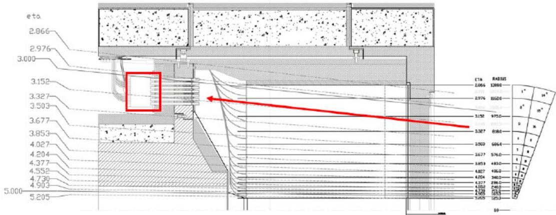
Figure 1. Diagram of HF. The red box is the PMT readout box, and the arrow indicates particles traveling from the interaction point.
