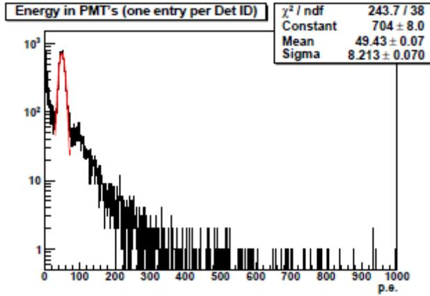
Figure 2. Energy in PMTs, 150 GeV muons.
