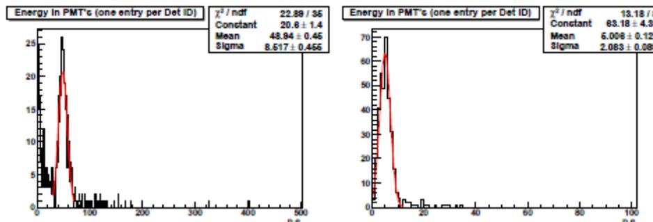
Figure 10. Energy in PMTs, 7 TeV minimum bias events, 6 mm window on left, 0.6 mm window on right.
