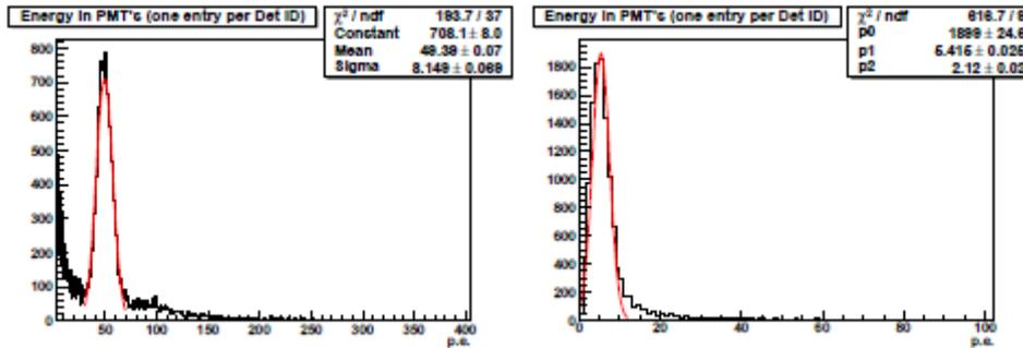
Figure 8. Energy in PMTs, 150 GeV muons, 6 mm window on left, 0.6 mm window on right.
