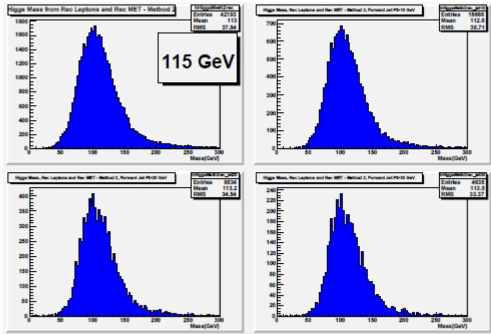
Figure 4. Results of forward jet cuts on Higgs reconstruction, 115 GeV Higgs. Top left, no cuts. The remaining histograms use the previous  $\eta$  cuts. Top right, jet  $p_T > 10$  GeV, bottom left, jet  $p_T > 20$  GeV, bottom left jet  $p_T > 30$  GeV.
