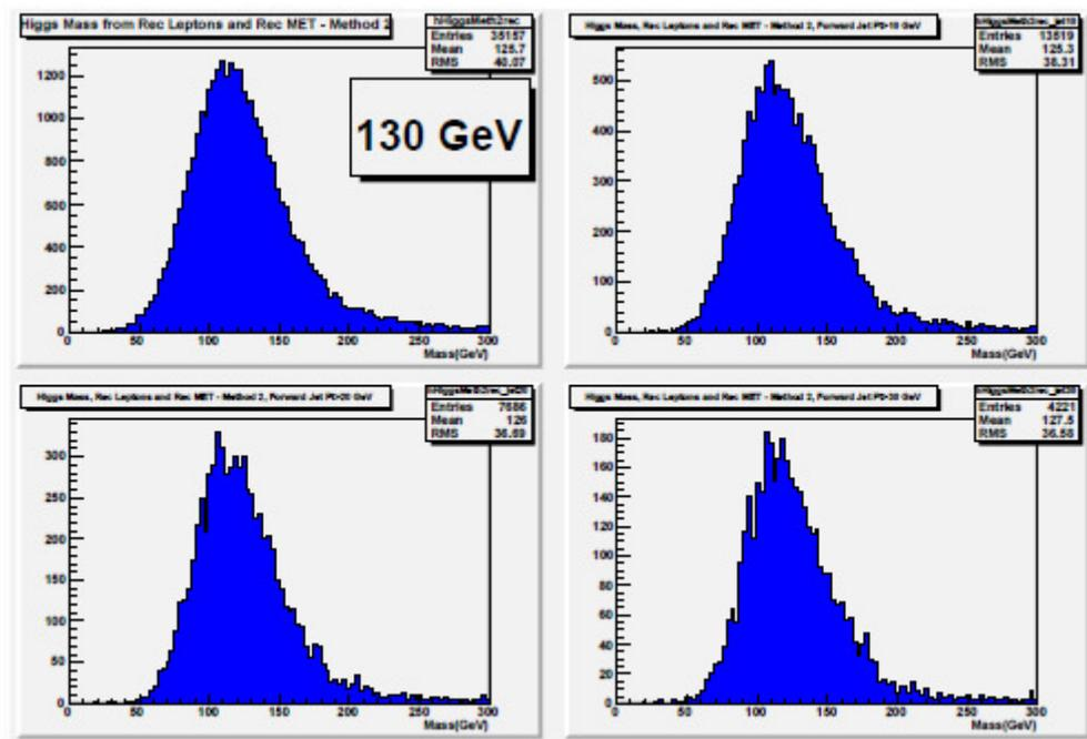
Figure 5. . Results of forward jet cuts on Higgs reconstruction, 130 GeV Higgs. Top left, no cuts. The remaining histograms use the previous  $\eta$  cuts. Top right, jet  $p_T > 10$  GeV, bottom left, jet  $p_T > 20$  GeV, bottom left jet  $p_T > 30$  GeV.
