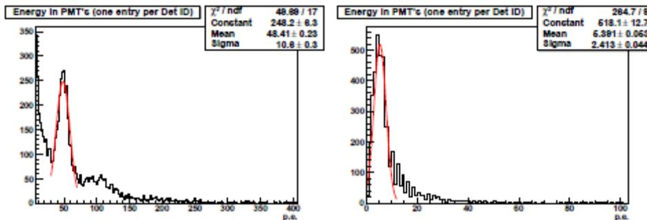
Figure 9. Energy in PMTs, 50 GeV pT Pythia jets, 6 mm window on left, 0.6 mm window on right.
