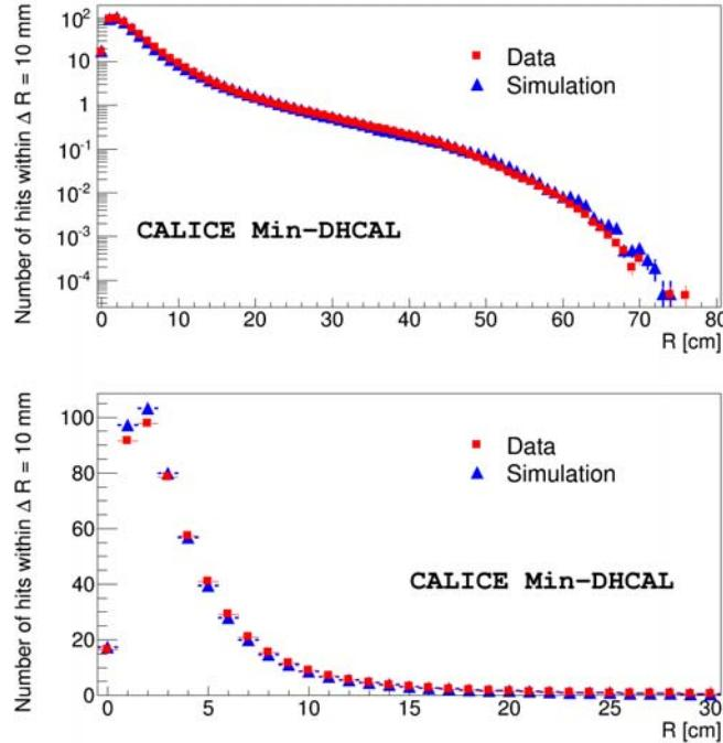
**Figure 4.** Distribution of the radial distance of hits from the shower axis for 6 GeV positrons. The upper (lower) plot uses a logarithm (linear) y-scale. The areas of both plots are normalized to one event. The error bars include the statistical and systematic uncertainties for the data and statistical uncertainties only for the simulation.
