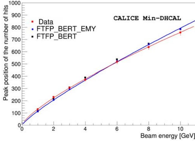
**Figure 2.** Peak position of the number of hits versus positron beam energy for both data (red) and simulation based on FTFP\_BERT (black) and FTFP\_BERT\_EMY (blue). The experimental data points and the simulation based on FTFP\_BERT\_EMY have been fitted to a power law shown as solid lines. The error bars of the data include both the statistical and systematic (dominant) errors. The statistical error bars of the simulation are smaller than the marker size.
