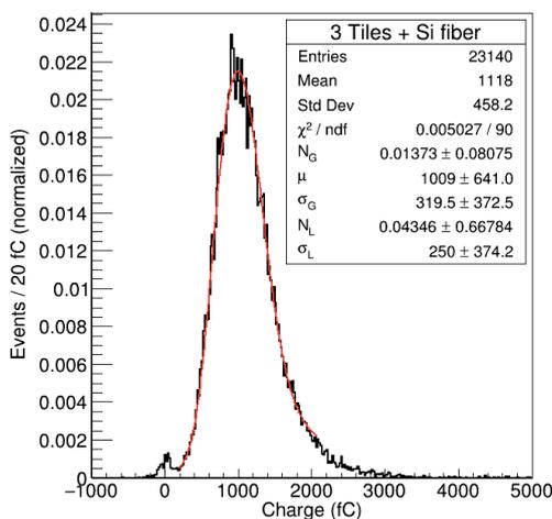
**Figure 5.** The response to traversing MIPs of the three-tile assembly read out with silicone-based WLS fiber passing through the center of the tiles and coupled to a SiPM.
