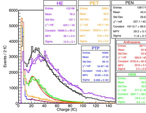
**Figure 1.** The response of the HE (reference scintillator tile: SCSN-81); PEN and PET tiles; stack of HEM sheets; quartz plates with pTp and anthracene coatings to 150 GeV muon beam.
