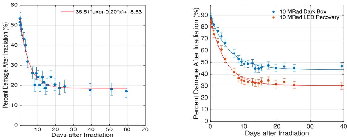
**Figure 4.** Radiation damage and recovery of PEN (left) and LED stimulated recovery of PEN (right).
