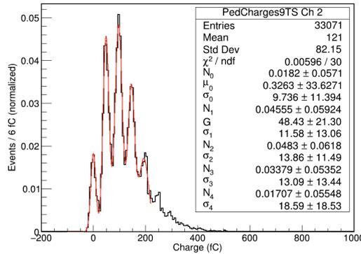
**Figure 2.** Pedestal charge spectrum of one of the photodetectors showing a few photon peaks.
