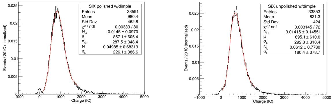
**Figure 3.** The charge spectrum of the new development of scintillators in response to traversing MIPs with polished (left) and unpolished (right) configurations.
