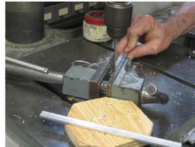
fit the edge for close contact with a photomultiplier tube (PMT). A “keeper” was formed to hold the plates in the frames. Plastic tubes were glued to the frames to
