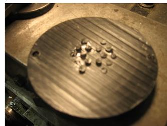
guides had to be in a pattern to match the photo-sensors to the fibers that brought the light from the calorimeter. The Quarknet group machined and polished the “cookie”-like device and delivered it to the detector group for evaluation.
