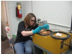
The group prepared 20 Quartz plates for test beam at CERN. These plates were coated with p-ter-phenyl at Fermi Lab to increase their Cherenkov light. The group polished the edge of the quartz plate and machined frames to
