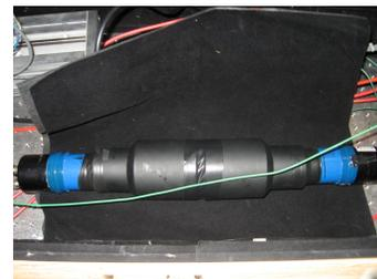
along the beam pipe that would measure background activity that would be fed into the main detectors as noise. This detector would discern the presence of muons and the direction
