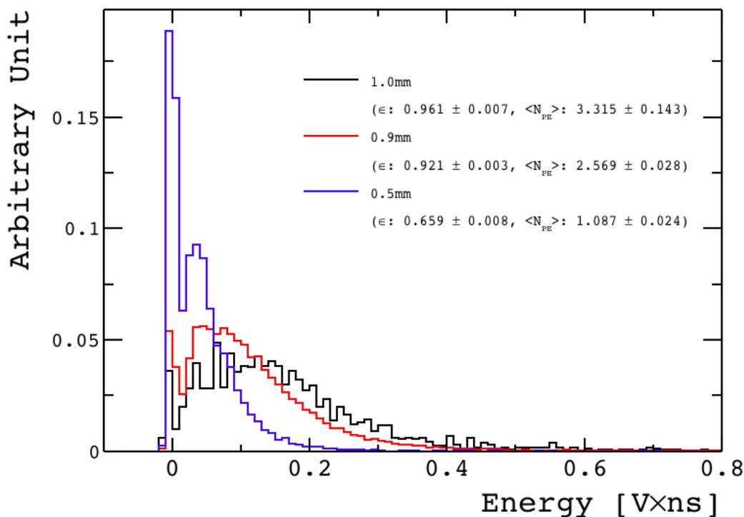
**Figure 5.** Comparison between the light output of liquid scintillator tiles readout with plastic WLS fibers with different thickness. The light output, proportional to the energy released by a particle traversing the scintillator volume, is measured in units of photodetector pulse area. The three distributions are normalized to have the same area of 1.
