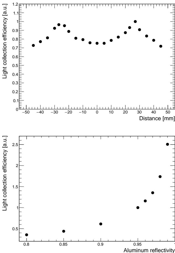
**Figure 7.** (Top) Ratio of light yield to maximum light yield from a simulated tile as a function of the distance perpendicular to the support tubes, normalized to the efficiency at the position of the support tubes. (Bottom) Light collection efficiency vs. aluminum reflectivity, normalized to a reflectivity of 0.95.
