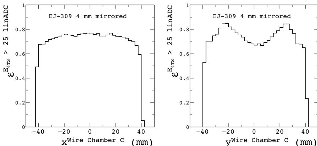
**Figure 2.** For the nominal liquid tile, fraction of muons with at least one photoelectron as a function of the impact position of the muon along the axis parallel to the support tubes (left) and perpendicular to the support tubes (right).
