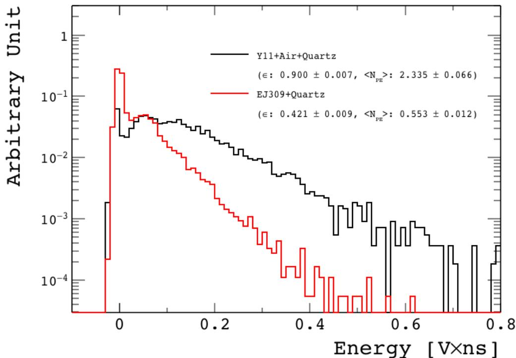
**Figure 4.** Comparison between the light output of a liquid scintillator tile equipped with a plastic WLS fiber, and a capillary filled with liquid WLS. The light output, proportional to the energy released by a particle traversing the scintillator volume, is measured in units of photodetector pulse area. The two distributions are normalized to unit area.
