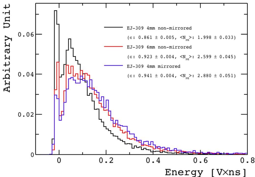
**Figure 3.** Comparison between the light output (arbitrary unit) of liquid scintillator tiles with different thickness and different treatment of the aluminum surface in contact with the liquid scintillator. The light output, proportional to the energy released by a particle traversing the scintillator volume, is measured in units of photodetector pulse area. The light is readout with the same 0.9 mm (O.D.) Y11 plastic WLS fiber. The three distributions are normalized to unit area.
