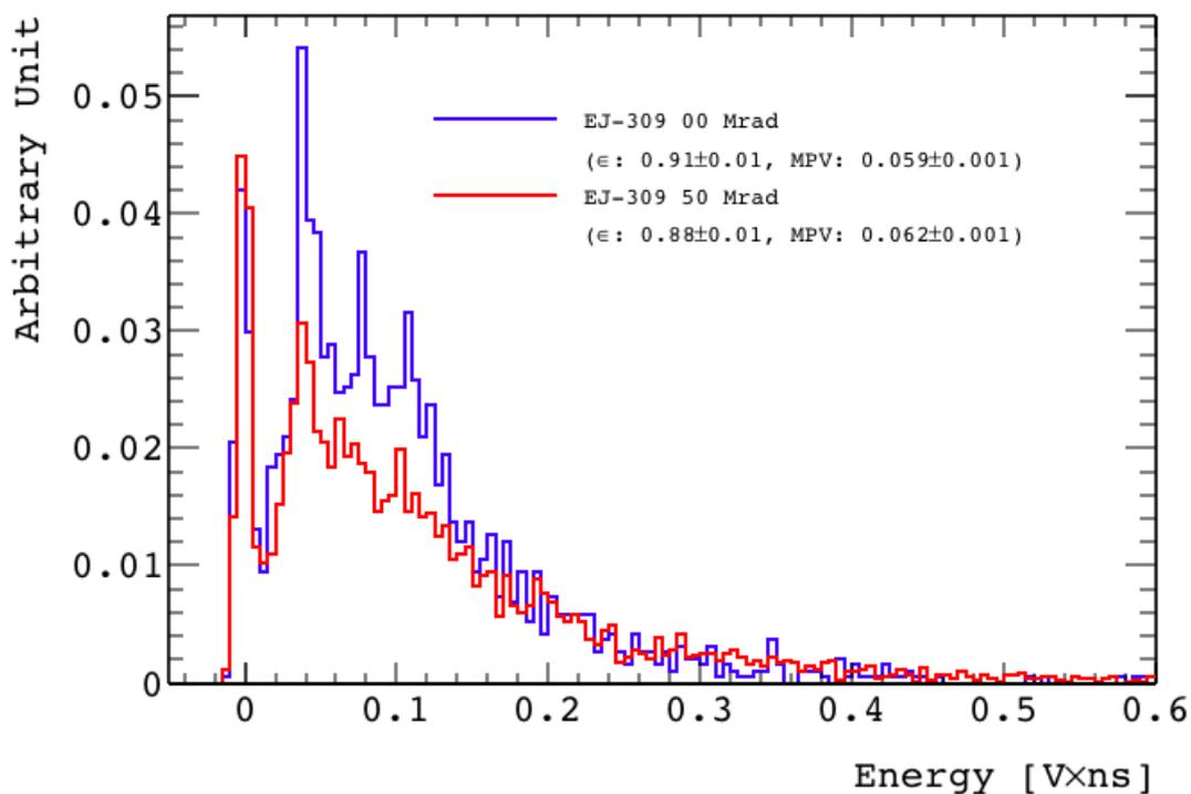
**Figure 6.** Comparison between the light output of a liquid scintillator tile filled with unirradiated (black) and irradiated (red) liquid scintillator. The light output, proportional to the energy released by a particle traversing the scintillator volume, is measured in units of photodetector pulse area. The two distributions are normalized to have the same number of events in the pedestal.
