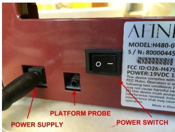
**Figure 1.3** Back of printer
