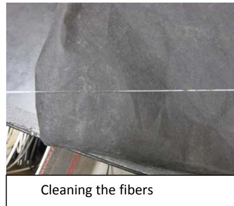
and pulling the fibers up against the pads. They rewashed the fibers with acetone to help reduce oils and fingerprints and inspected them to ensure that they had not been scratched and had all possible dirt and plastic removed.
