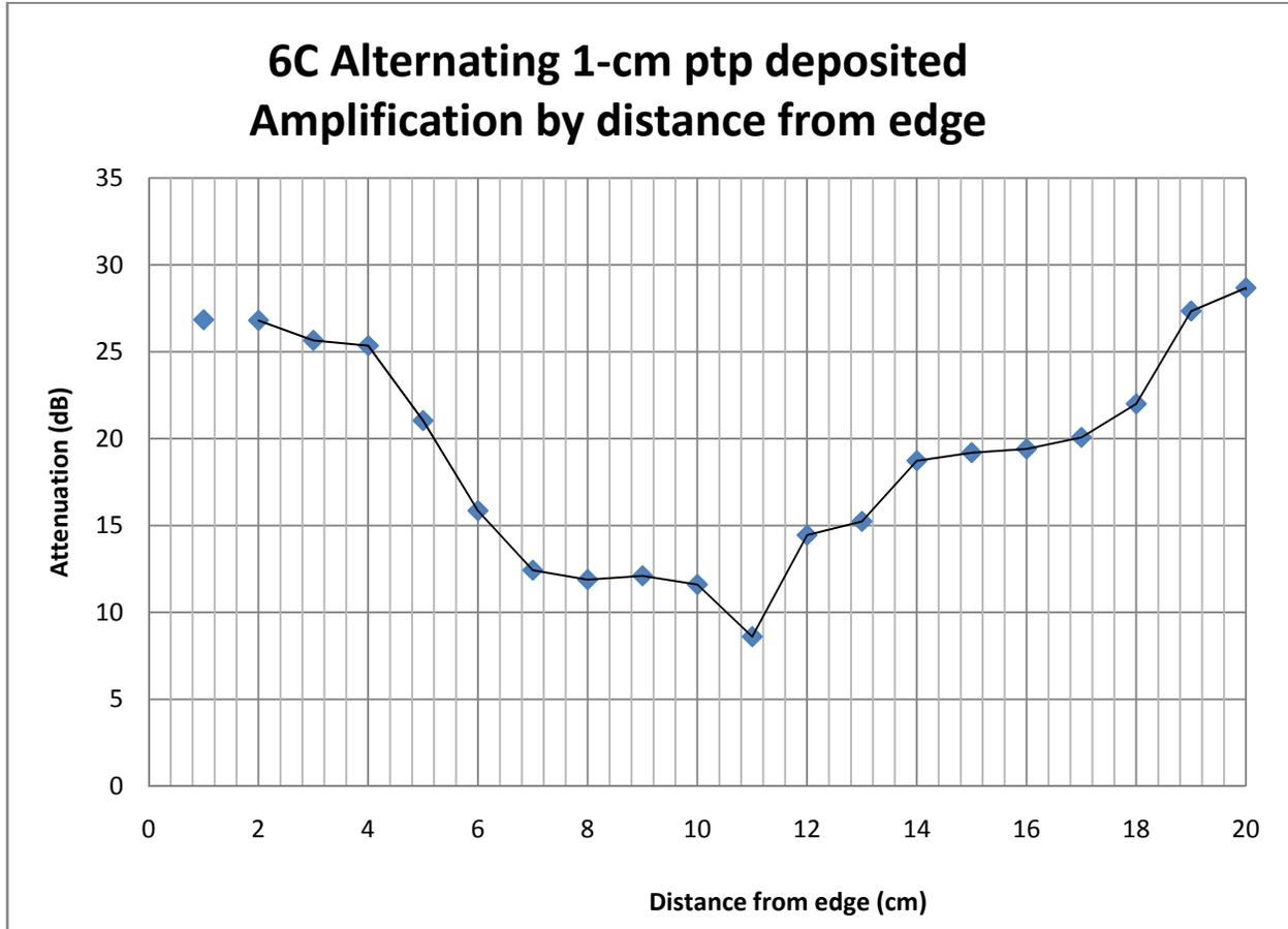
This graph shows the distribution of attenuation over the distance edge-to-edge for the 1 cm-staggered treatment. It appears to have higher signal than the bare 20 cm width but still suffers from loss in the center but to a lesser degree.
