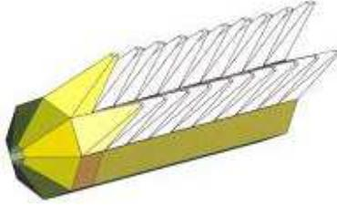
**Fig. 2.** Schematic of CASTOR showing two rows of internally reflecting air light guides. The interaction point is to the left.
